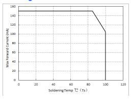
Max Driving Forward Current vs. Soldering Temp
