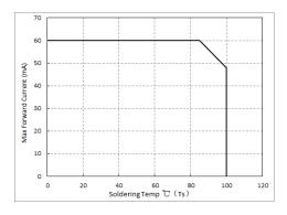
Max Driving Forward Current vs. Soldering Temp
